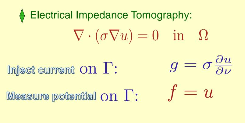
**EIT:** given (f, g), recover electrical conductivity  $\sigma(x)$
